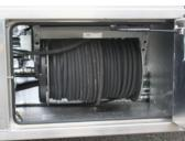
wand, delivering a high pressure stream to break up material. A self-wind reel has 75 feet of high pressure hose, while an optional hose reel has up to 350 feet of high pressure hose.
