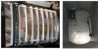
Rugged debris bodies that are built to last An oval shape with cylindrical sides creates extra strength and efficient material dumping. Powder coat paint creates a heavy-duty, durable finish, while the optional galvanized tanks carry a lifetime warranty.
