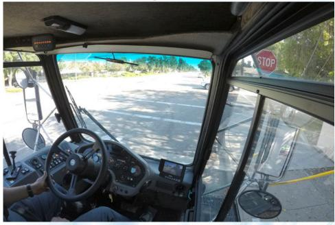
**THE BEST TURNING RADIUS & EXCEPTIONAL VISIBILITY** With the center mounted cab/forward layout the operator has unsurpassed visibility of the road surface as well as pedestrians and surrounding traffic. The 116-inch wheelbase allows for the sweeper to reach a **turning radius of 12 1/2', wall-to-wall**. With the pickup Head in the center you don't have to worry about what is happening behind you. The **Global R3AIR**'s exceptional visibility increases operator and pedestrian safety.
